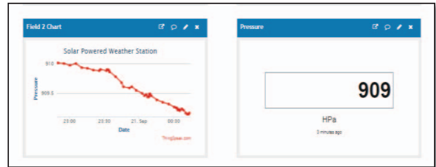
Fig. 5. Pressure Vs Time Plot (ThingSpeak)
