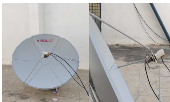
Fig. 24: POTY feed antenna and LNB mounted on the dish
