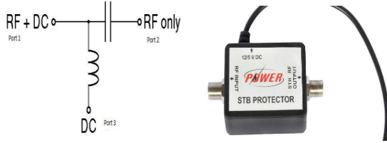
Fig 8: Working of Bias-T Fig 9: 3 Port 12V Bias-T
