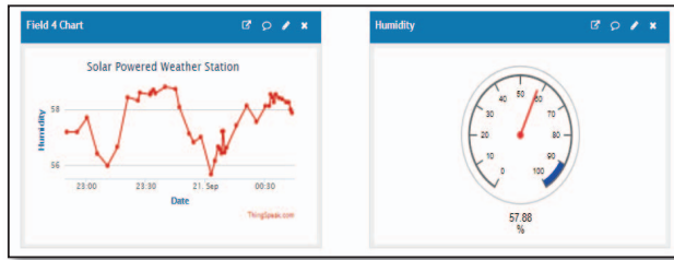
Fig. 7. Humidity Vs Time Plot (ThingSpeak)
