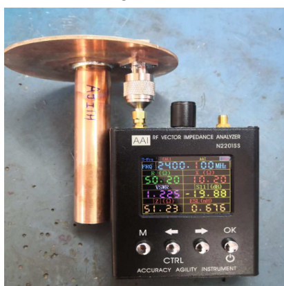
Fig. 23: POTY feed antenna testing using VNA
