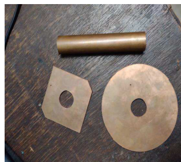
Fig. 21: Materials used for constructing the antenna
