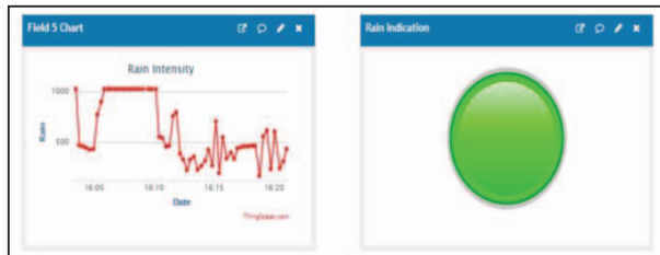
Fig. 9. 1/Rain Intensity Vs Time Plot (ThingSpeak) (Raining Condition)
