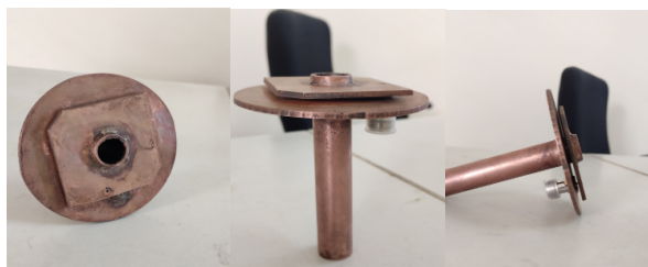
Fig. 22: The final design of the POTY feed antenna
