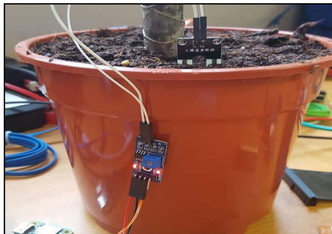
Figure 4. Soil water potentiometers for measuring the matric potential (courtesy: Soil water movement procedure by H.Horde)
