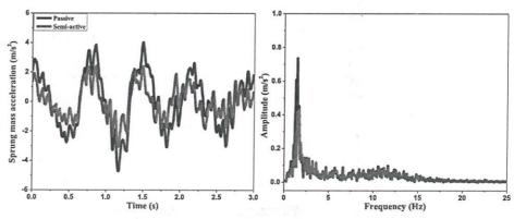
Dynamic analysis has been carried out by using quarter car model with passive and semi-active
