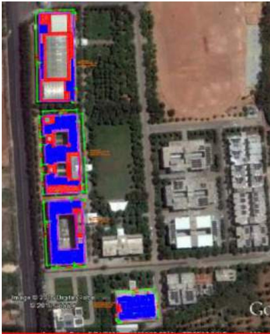
Figure 40: Free roof top available for solar PV at REVA University .
